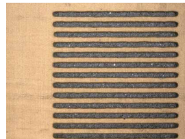
Print after 1 hour wait (180 µm)
